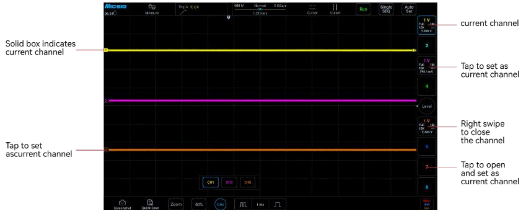
Figure 5-4 Channel Open, Close and Switching
